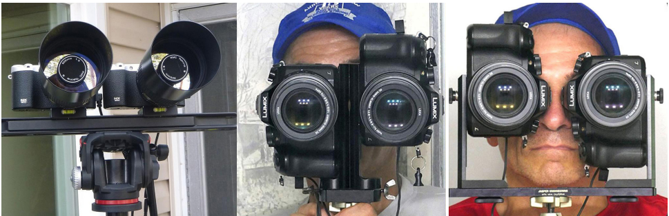
Three possible twin camera arrangements: 1) Side-by-side (left) is the simplest arrangement, but difficult to use in the field. 2) Bottom-to-bottom (center) is easier to align and carry around. 3) Top-to-top (right) has the advantages of #2 with the extra benefit of composing in 3D.
