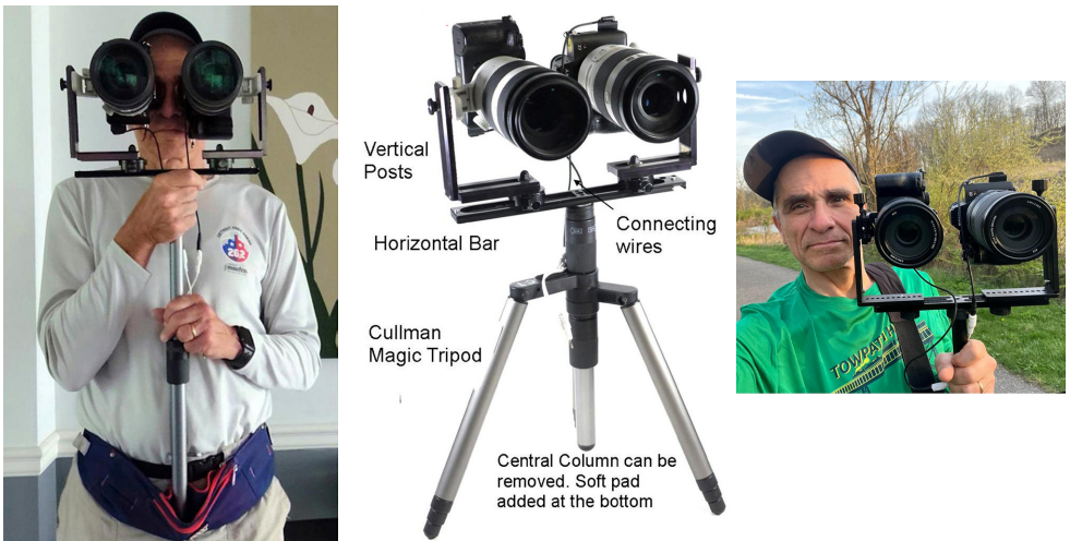
My wildlife 3D rig (see Text for details). The heavier 100-400 mm lenses are on the left and center, and the lighter 75-300 mm lenses on the right.
