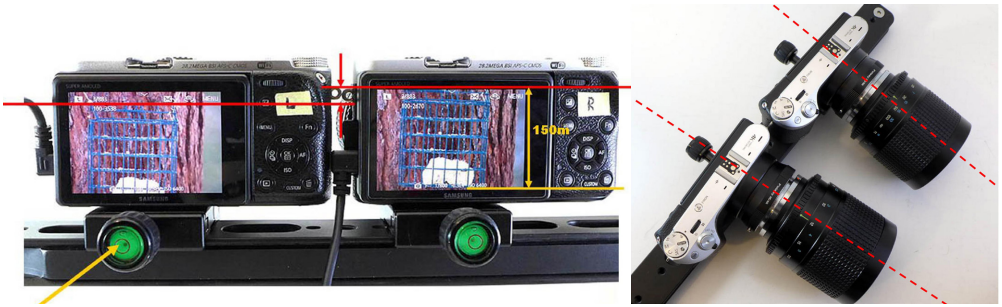
Left: Even though the cameras and mounts are identical, the left camera is lower than the right camera. The high magnification magnifies any vertical error. Right: The cameras must converge to the main subject to minimize image loss and allow the use of auto focus.
